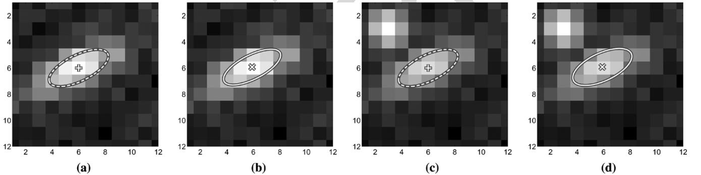
Fig. 3. Examples with 2-D synthetic data. (a), (b) Ground-truth and our method's estimate for an anisotropic Gaussian  $\Sigma = [2 \ -2; -2 \ 5]$  with random additive noise. (c), (d) Those for two Gaussians with the noise. The center of the smaller Gaussian is deviated by 2 Mahalanobis distance away from the target Gaussian. "+" and dashed-ellipses indicate ground-truth local maximum and spread. "x" and solid-ellipses display those estimated by our 2-D algorithm.
